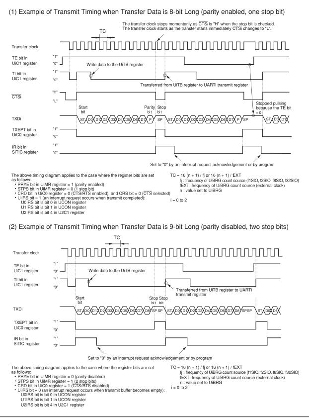
Figure 14.17 Transmit Operation
